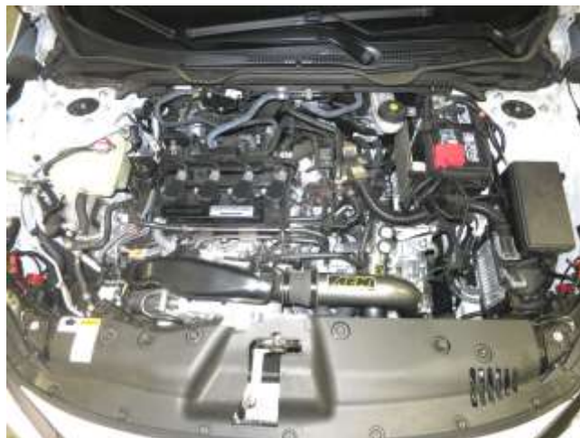
AEM CHARGE PIPE INSTALLED
