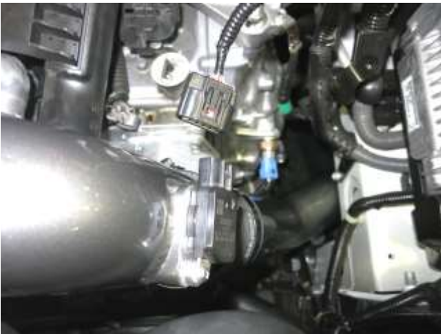
a. Disconnect mass air flow (MAF) sensor harness.
