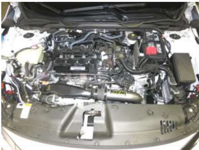
STOCK CHARGE PIPE INSTALLED
