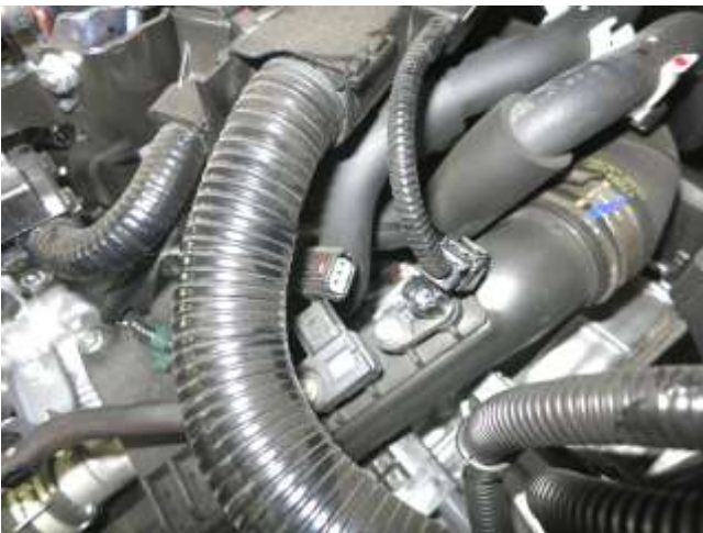
c. Disconnect the manifold absolute pressure (MAP) sensor and intake air temperature (IAT) sensor harnesses.
