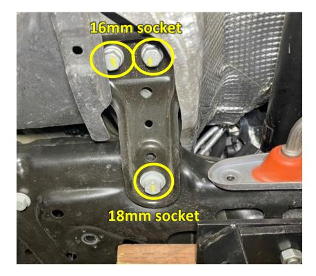
13F Undo subframe bolts with a (18mm socket).
