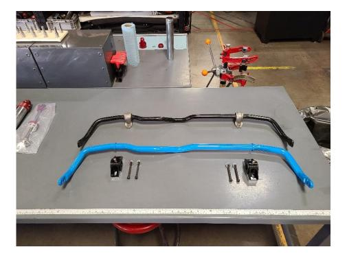
16F Install the front aFe Control sway bar in the same manner as factory removal. We suggest leaving the sway bar in the poly bag when feeding it into the car. This will keep it safe from scratches. (remove poly bag once bar is in place)
