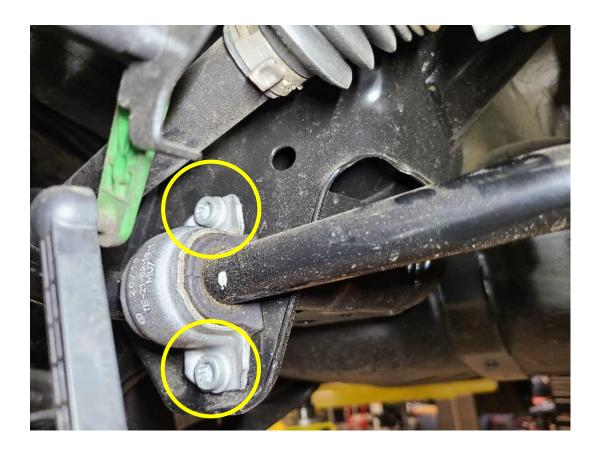
9R Lower the exhaust slightly and remove the factory sway bar from the vehicle. Note the orientation of the sway bar when removing. (i.e. observe which is the top of the sway bar and how the ends are pointing.)
