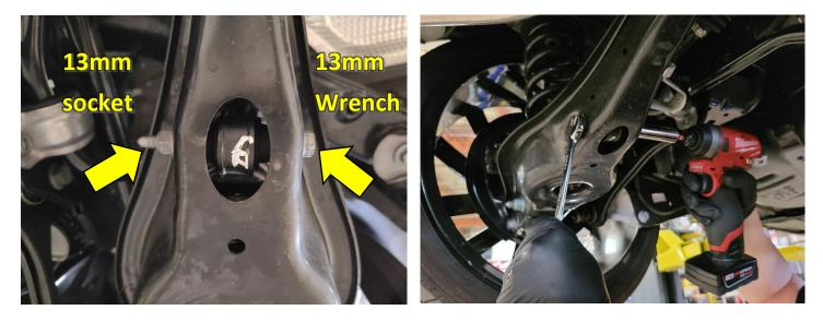
8R Remove the bushing brackets with a (M10 Triple Square).
