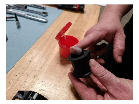
13R Install the bushing onto the sway bar. The bushings should be positioned just outside of the centering rings. Slide the aFe Control bushing bracket onto the bushings and mate the sway bar assembly to the subframe as shown in the diagram. Fully tighten this hardware to factory specs.
