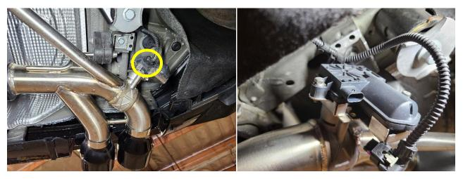
4R Remove the exhaust rear hanger bolts (2) with a (13mm socket).
