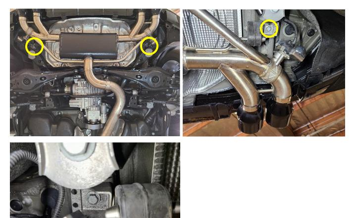
5R Unbolt the center brace with a (13mm socket).
