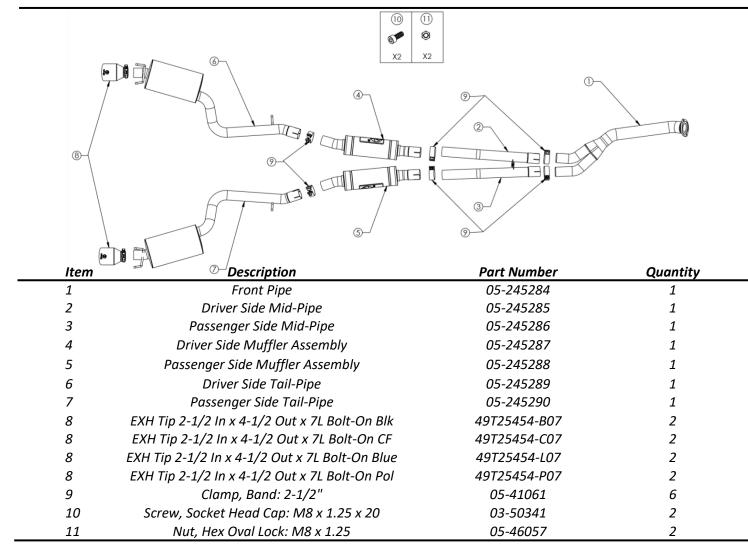
**aFe POWER recommends professional installation on this product.** Thoroughly inspect the aFe POWER exhaust system to make sure there is no damage from shipping (if damage is noted, immediately contact aFe POWER customer service). Allow time for your vehicle to cool down prior to installation. When working on your vehicle proceed with caution. Wear protective safety equipment; eye goggles and gloves to ensure a safe installation.
