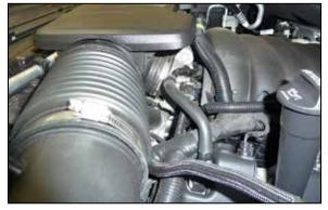
3. Loosen the two hose clamps that secure the intake plenum to the throttle body and the air filter housing and then remove the intake plenum from the vehicle.
