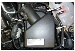
Loosen the three screws that secure the air filter housing lid and then lift up the housing and set aside.
