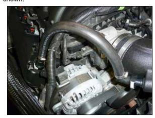
11. Install the crank case hose assembly onto the quick connect fittings on the intake tube and valve cover as shown.
