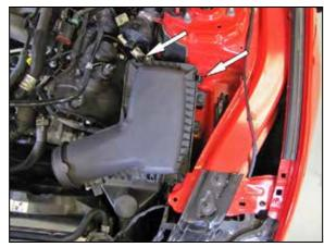
8.Release the two clips that secure the upper air filter housing and remove the upper housing from the vehicle.
