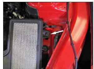
9. Remove the bolt that secures the lower air filter housing to the inner fender and then remove the lower housing from the vehicle.
