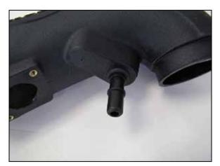
12. Install the large quick disconnect fitting into the AIRAID<sup>®</sup> intake tube using the provided grommet.
