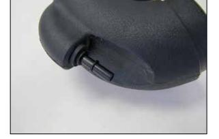
11. Install the small quick disconnect fitting into the AIRAID<sup>®</sup> intake tube using the provided grommet.
