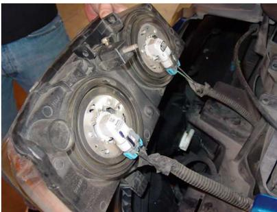
Step 5: connect the wire harness to the new anzo headlight. Bulbs are supplied with the headlight.
