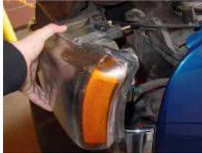
Step 3: Pull the headlight straight out of the housing.
