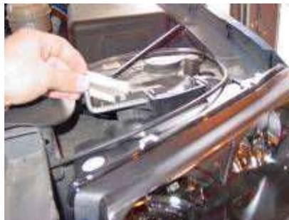
Step 6: install the headlight back into the housing, slide the pin back in place.
