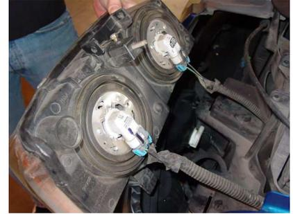
Step 4: Disconnect the headlight wire harness from the high and low beam light bulbs.
