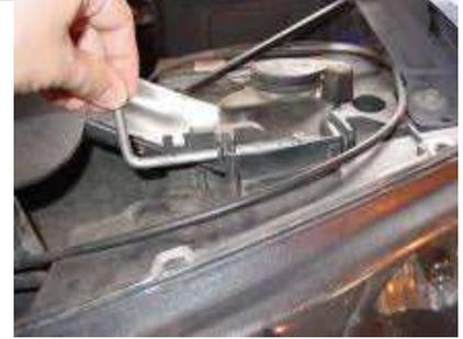
Step 2: Pull the pin straight out to loosen the headlight assembly.
