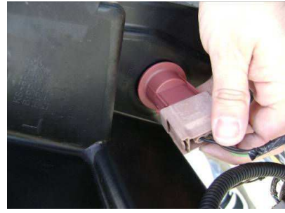
Step 17: plug the inner marker harness to the socket .
