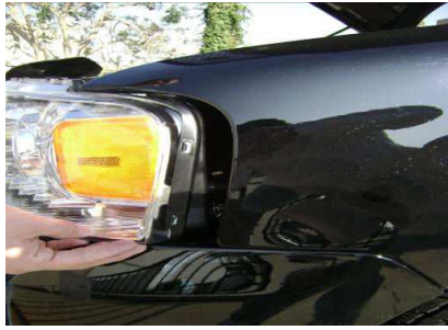
Step 19: Place the headlight assembly into the headlight housing.
