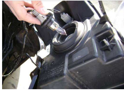
Step 7: Twist and pull the headlight bulb out of the housing.
