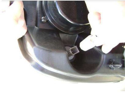
Step 16: Plug the side maker harness to the socket.
