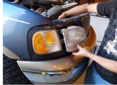
Step 3: Pull off the headlight assembly straight out from the car and unplug the headlight harness.
