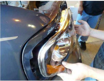
Step 10: Align the headlight and place back into housing.
