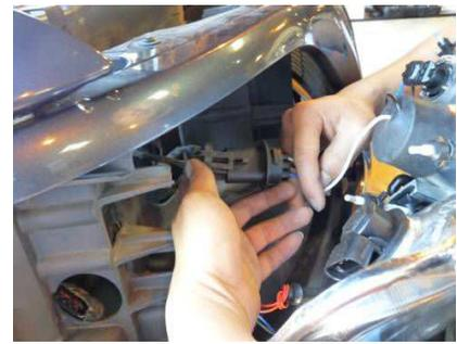
Step 7: Splice in the halos into the corner light. Halo wires are two red one power and the other wire ground. Splice one red wire (+) positive into the brown wire on the corner light. Other red wire (-) negative will be spliced into the black wire on the corner light.
