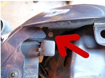
Step 4: Use the t20 torque screw to remove the screw holding in the corner light. Located at the top of the corner light
