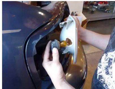
Step 5: Remove the bulb from the corner light.
