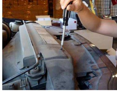
Step 1: Remove the eight plastic screws holding in the plastic cover shroud.
