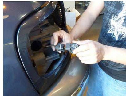
Step 6: Remove corner bulb out from the harness.
