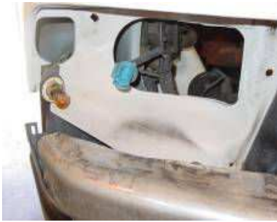
Step 9: Remove the headlight from the car.
