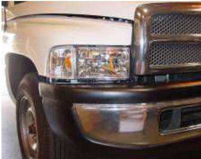
Step 12: Bolt on the headlight and check all functions before driving.
