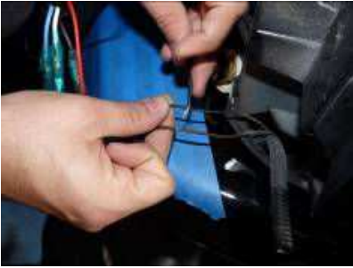
Step 13: Splice the black (-) wire into the black wire of the parking light to light up the leds.
