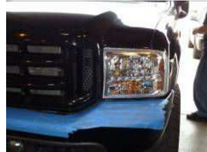
Step 15: Twist in the parking and signal light into the new Anzo head light.
