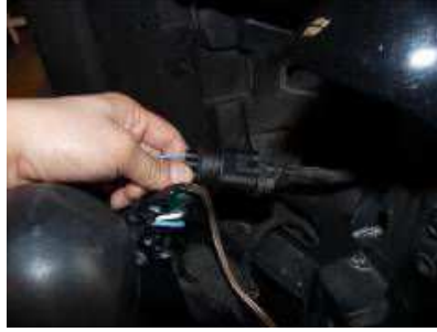
Step 14: Plug in the head light wire harness into the new Anzo light.
