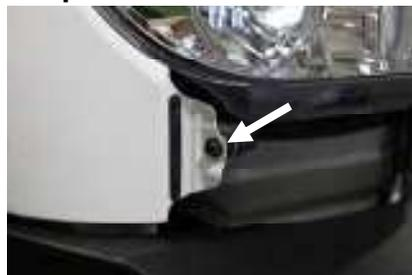
Remove the 10mm screw located at the bottom of the headlight housing
