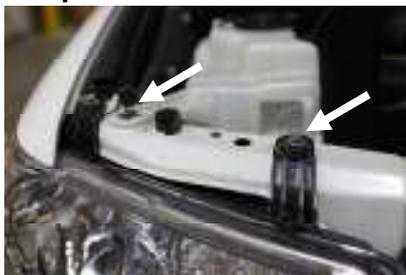
Remove the two 10mm screws located at the top of the headlight housing
