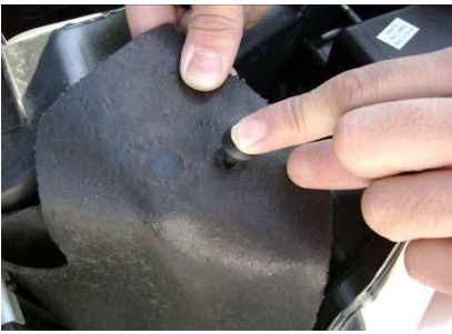
Step 21: Place the plastic clip back in place.
