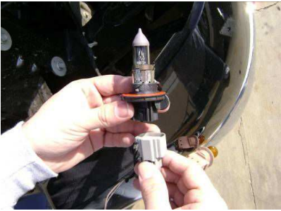
Step 9: Disconnect the headlight bulb from the wire harness.
