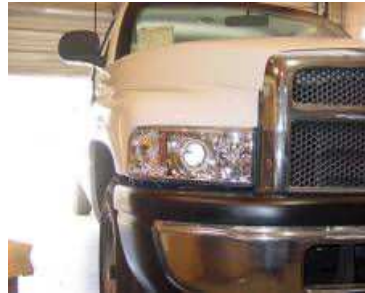
Step 15: Bolt on the headlight and check all functions before driving.
