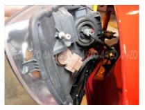
Step 5: Remove the head light from the vehicle.
