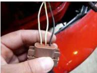
Step 10: For 2007-2008 trucks you will have to splice the halos. Pull back the cover to expose the wires on the corner parking light.
