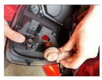
Step 13: Twist the corner parking into the new head light.
