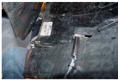
Step 10: Remove the 10mm screw holding in the lip to the bumper cover.
