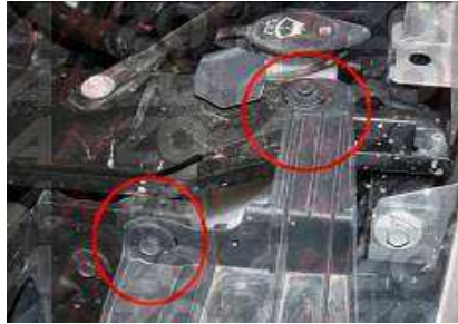
Step 13: Remove the two 10mm screws holding the headlight in place.
