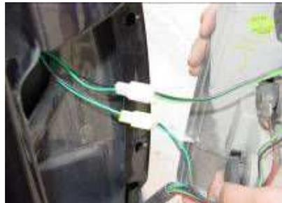
Step 7: plug the two resistors into the tail light.
