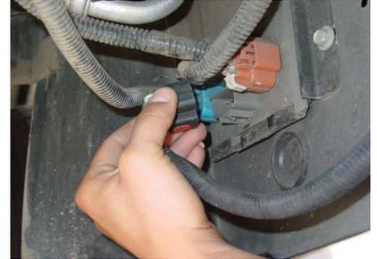
Step 2: Unplug the middle wire harness from the circuit board.
