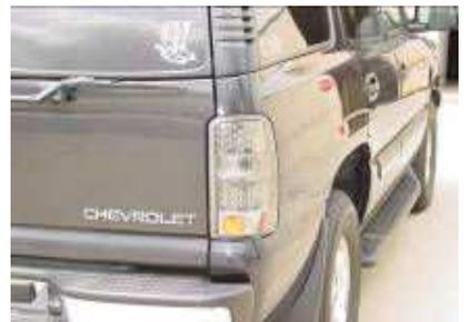
Step 8: Put the tail light in and screw in the two screws to hold the tail light in place.
