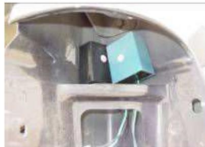
Step 6: Remove the protective sticker backing from the resistors and stick them inside the top tail light housing.
