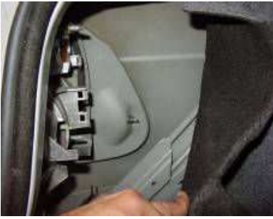
Step 10: Pull back the trunk lining to remove the last bolt.
