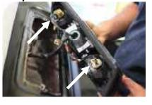
Insert the reverse light bulb sockets into the Anzo third brake light housing
