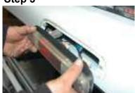
Carefully pull out the OEM third brake light housing from the vehicle.
