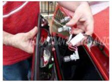
Step 3: Twist off the light bulb socket from the third brake light.
