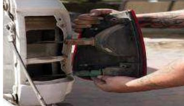
Once the 2 bolts are removed pull the taillight off the body and untwist the light sockets from the housing.
