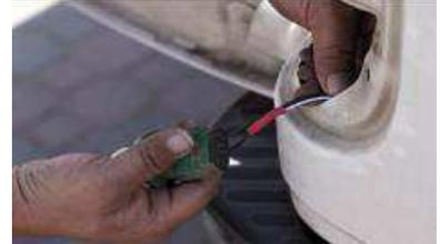
Route the white wire up through the taillight pocket from the underside of the vehicle. This wire gets connected to the power wire on the reverse bulb. In this case the wire was black with a red tracer. Once this is done replace the taillight back on the vehicle.
