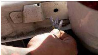
There is a hole in the tailgate located on the bottom passenger side. This is where you will run your wires through.
