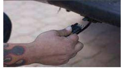
Route the harness with the flat 4 connector behind the bumper and connect it to your trailer wiring.
