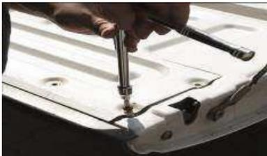
You will need to remove the torx bolts holding the panel on the back of your tailgate.
