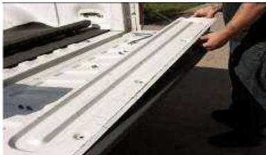
Once the torx bolts are removed lift the panel off of the tailgate.
