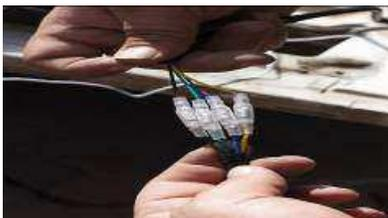
Once you have all the wires through you can connect them to each other by matching up the colors. The white wire will be wired into the taillight so make sure this is coming out the bottom of the tailgate.
