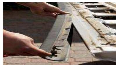
Remove your stock cap by pulling up from one corner. The cap is held in with clips so you may need to use some force to get it started.
