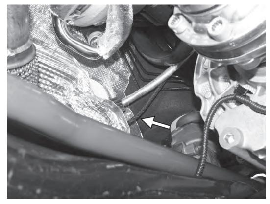
95) Connect the APR extension harness to the secondary oxygen sensor connector. Fold and tuck any excess cabling behind the center tunnel heat shielding.
