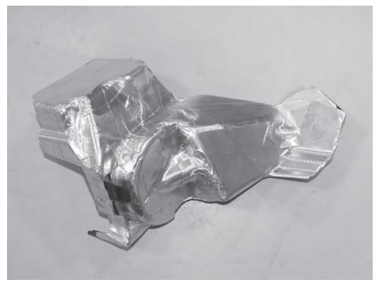
41) Remove the plastic heat shield from the ABS brake pump that is located on the lower right side of the engine firewall. Cover the outside of the heat shield with the supplied heat reflective tape. Reinstall the cover to the ABS brake pump.
