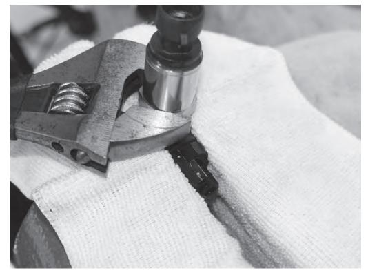
73) Unscrew the two portions of the APR boost tap. Carefully mount the main body of the boost tap in a bench vice with rags to protect the finish, being careful not to bend or crush the barbed fitting. Apply the supplied thread sealant to the threads of the APR boost sensor, and then install in the APR boost tap. Tighten the sensor with an adjustable wrench.
