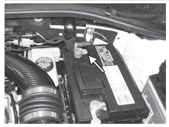
1) Disconnect the 10mm negative battery terminal and set aside. Remove the engine cover from the top of the engine by lifting up on the corners of it.
