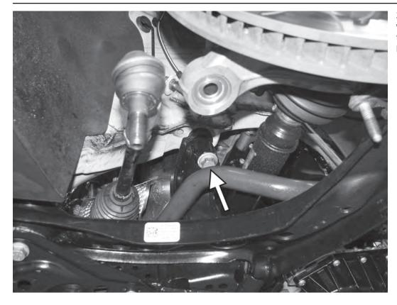
23) Remove the two 18mm bolts where the upper subframe meets the frame rail. As you remove these bolts, the subframe will slightly lower.
