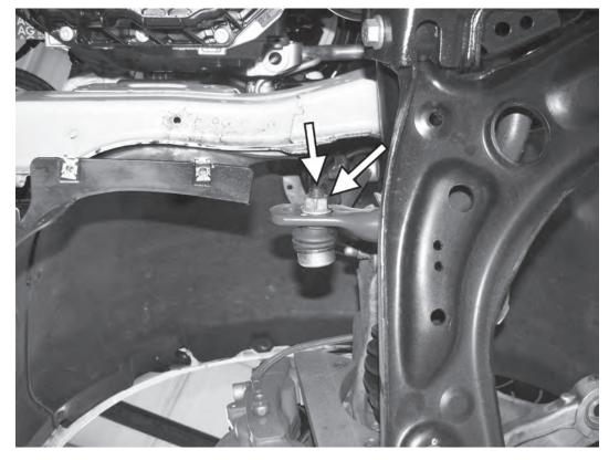
19) Use an 18mm wrench to separate the sway bar end link. If necessary, counterhold the end of the screw with a 6mm triple square.
