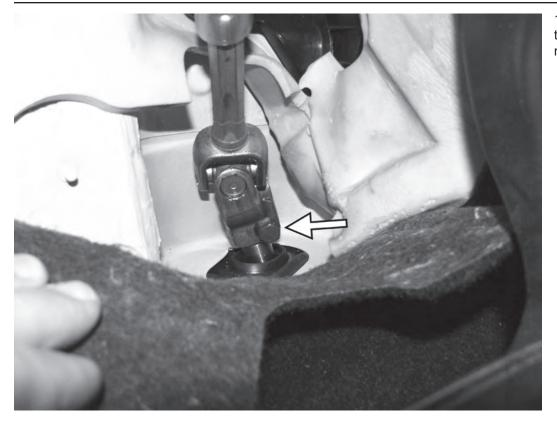
15) Remove the 13mm bolt holding the steering column to the steering rack.
