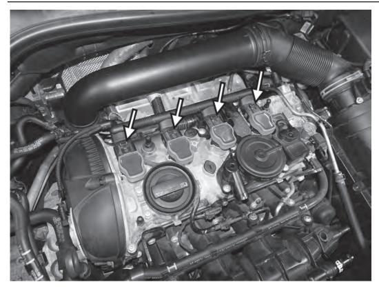
3) Disconnect the four electrical connectors to the ignition coilpacks, and lift the harness away from the coilpacks.
