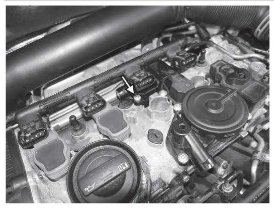
9) Reinstall the plastic connection piece into the oil separator, and secure with the original T30 screw.
