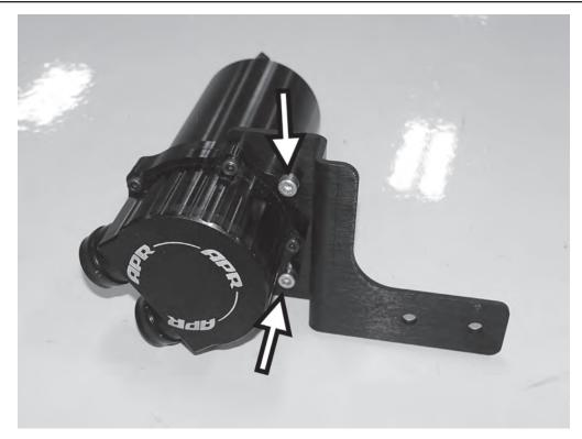
11) Mount the APR bracket to the APR catch can with the two supplied 4mm allen screws.
