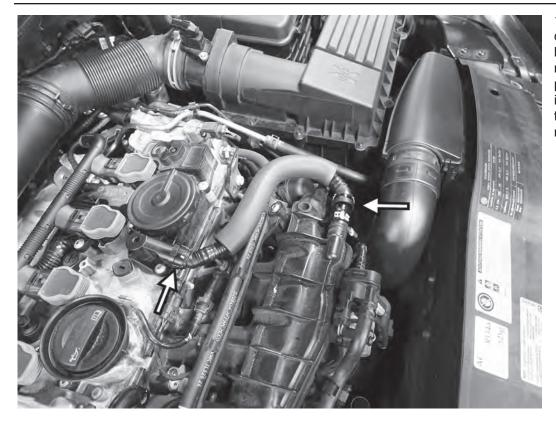
1) Remove the engine cover. Disconnect the vent line that goes between the valve cover and intake manifold. Once removed, install the plug supplied with the APR boost tap in the boost tap with thread sealant to close off this port on the intake manifold.
