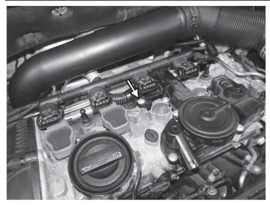
5) Remove the T30 screw from the vent line that connects to the oil separator on top of the valve cover.
