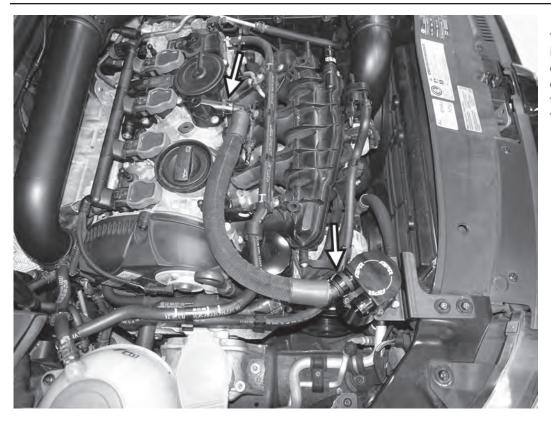
13) Lubricate the fitting o-rings on the shorter APR catch can hose, and install between the port on the front of the valve cover and the left port of the APR catch can. Simply push the Norma connections in place until they click.
