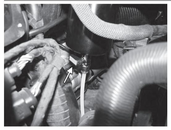
15) Confirm that the drain valve on the catch can is closed (parallel to the ground). The catch can can be drained by holding a cup under the drain valve and opening it.
