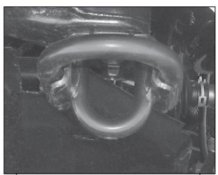
(Fig 8) Temporarily remove tow hooks. Important, the heavy duty factory tow hooks (pictured) cannot be reinstalled.
