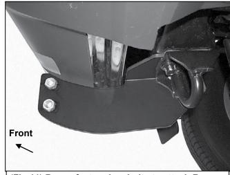
(Fig 11) Reuse factory hex bolts to attach Frame Bracket to bottom of frame (passenger/right side pictured with small tow hook)
