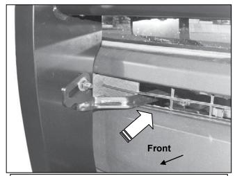
(Fig 18) Passenger/right Top Bracket installed
