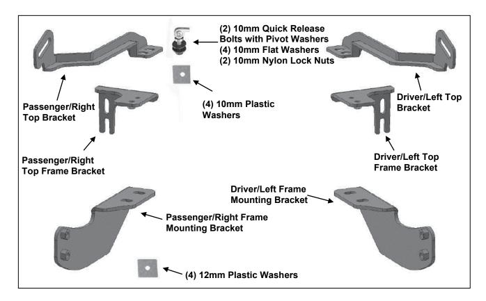
IMPORTANT: The Grille Guard is designed to tilt forward to clear the attached grille on 2007-13 Tundra, 08-14 Sequoia models. To tilt the Grille Guard, the Quick Release Bolts on the Top Brackets must be released and the upper bolts on both Mounting Brackets may need to be loosened slightly. Make sure that all hardware is fully tightened after closing the hood. Carefully read Page 8, "Opening and Closing of Hood," before installing the Grille Guard.
