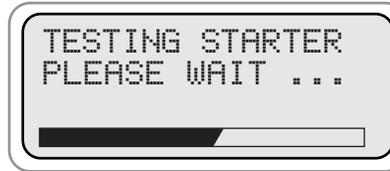
The BVA-300 will test the starting system. A bar at the bottom of the screen will show the tests progress.
