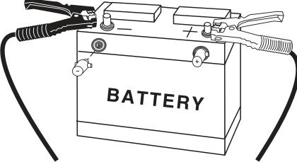
Note! Take special care when connecting to battery side terminals. If necessary use a side post adapter to prevent thread damage. When testing dual post batteries always connect load clamps to the post to which the system is attached.
