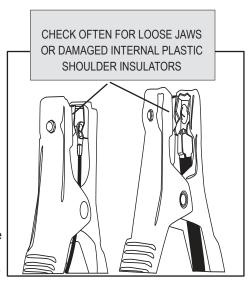
Over time the battery clamps will need to be replaced if any of the following are indicated:
