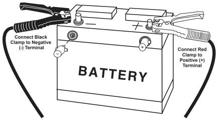
Note! Take special care when connecting to battery side terminals. If necessary use a side post adapter to prevent thread damage. When testing dual post batteries always check the post to which the system is attached. If a load test is made from a post connection and the alternator is mounted to side terminals a battery load test can be completed, but a continuity problem may still be in the side terminals when testing the alternator.
