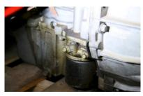
• Before removal, observe, or mark on this part, where you have ample clearance for the sender or pressure line. If there is no room for a sender due to aftermarket headers, you may then use a stainless steel line kit, such as an Auto Meter 3227 to remotely mount the sender.
