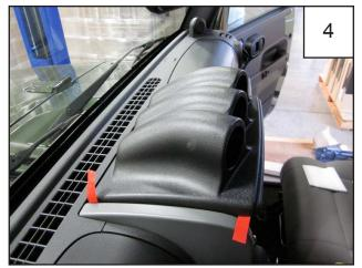
It is recommended that you align the part on the dash an equal distance between the front and the back edges. *NOTE: Alignment between front and back edges is adjustable based on customer discretion.*
