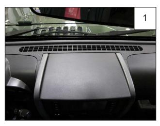
Clean all dirt and debris from dash. Dry fit the pod on the dash, and determine how you will run your gauge wiring. This pod can be used with or without gauge brackets. If no brackets are used, you can leave the gauges out until the pod is mounted, however wiring must already be in place and easily reachable. If you chose to use gauge brackets must already be mounted and wired before mounting the pod.
