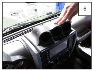
Apply firm pressure for 30 seconds on each section of the part to ensure proper adhesion.
