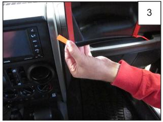
*Gauges must be installed in the triple gauge pod prior to installation.* Before placing the part on the vehicle, take the tabs for the line of 1/2" tape on the front and back of the part and fold it out as shown.
