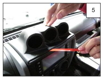
Pull liner of lower 1/2" tape strip. Press down on entire length of the part again applying firm pressure to the taped areas. *NOTE: The tape reaches maximum adhesive bond after 24 hours of contact.*
