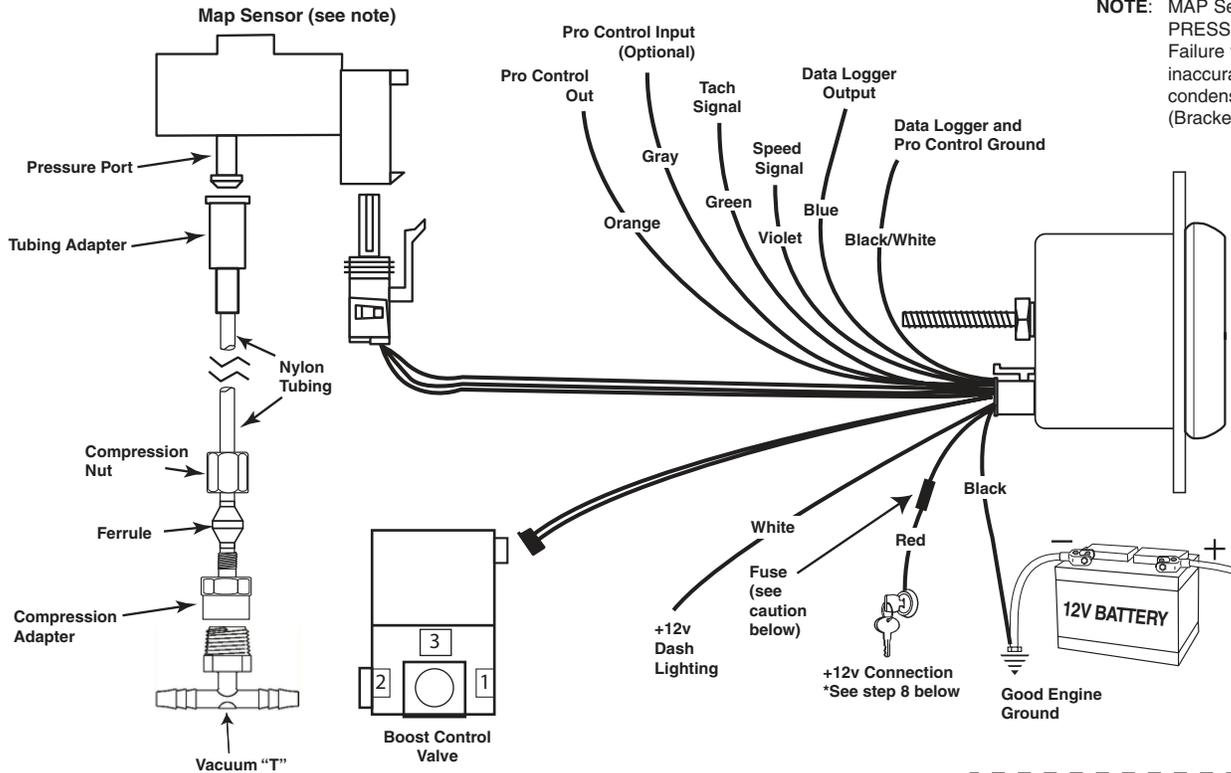
**NOTE:** MAP Sensor should be mounted with PRESSURE PORT facing down. Failure to do so could result in inaccurate readings due to condensation in the line. (Bracket fabrication may be required.)
