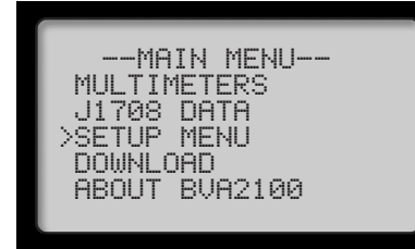
From the main menu scroll to the bottom and select SETUP MENU
