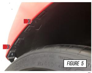
Pull back the wheel liner and remove the 2 torx screw (**A**) and the 1 nut (**B**) per each side, shown in **Figure 6**, with the bumper already removed.
