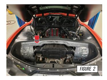
Spray the both the driver and passenger side flange with penetrating oil, to aid in removal. Let the penetrating oil soak while removing the bumper.
