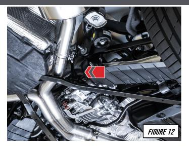
It is crucial to install each section and Accu-Seal clamp correctly to prevent loose joints and exhaust leaks between the tubing connections.
