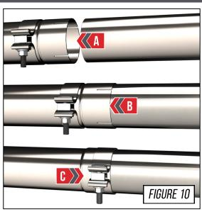
After the *1FG* system has been properly installed in the factory exhaust hangers, and adjusted; begin torqueing the forward most clamps and bolts, then move gradually towards the rear of the vehicle, properly torqueing each clamp along the way, as shown in **Figure 11**.
