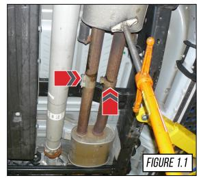
Loosen the clamps just after the muffler, located above the rear axle; as shown by the arrows in **Figure 1.2**.
