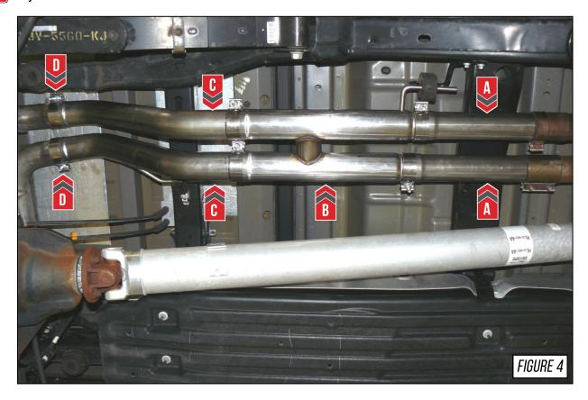
It is crucial to install each section and Accu-Seal clamp correctly to prevent loose joints and exhaust leaks between the tubing connections.
