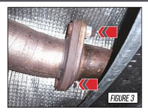
Install the resonated front section (part **YO**), reusing the factory gasket and supplied M8 hardware.
