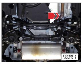
Cut the exhaust at the area located just after the welded joint, shown by the arrow in Figure 1.
