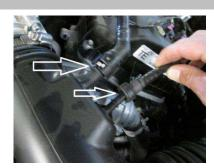
Disconnect the 2 breather hoses from the inlet tube. Loosen the clamps on the inlet tube at the throttle body and the air box, remove the inlet tube from the vehicle.
