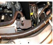
Remove the 2 10mm bolts from the driver side radiator mount and remove the mount by pulling it upwards from the vehicle. Install the BBK Air Filter Shield into place by setting it straight down onto the radiator mount peg. Install the stock bolt thru the air shield and bolt it back into the small tab on the inner fender. Reinstall the upper radiator mount and tighten the 2 bolts.
