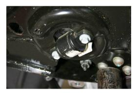
D. Loosen the top nut securing the top of the shock to the frame using an 18mm socket.
