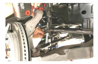
C. Loosen the two lower shock bolts holding the shock bar pin to the lower control arm with a 13mm socket.
