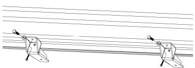
6. Place the Front Mounting Brackets back into place. With the Blind Retainer Nuts installed, use the 5/16" X 1" bolts with the flat washers and tighten both brackets to the vehicle. Take the two ¼" self-tapping screws and install them through the ¼" holes on the top of the Front Mounting Brackets. An impact wrench will make this easier.
