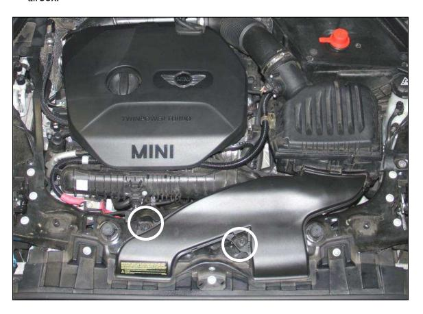
5. The pressure sensor is indicated below. It will have a connector that is identical the ones on the DINANTronics SPORT module.
