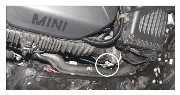
6. Disconnect the wiring harness from the pressure sensor.
