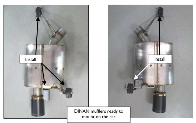
5. Place exhaust clamps provided in the hardware kit onto the ends of the stock exhaust pipes. With one of the DINAN mufflers secured on a jack or stand, put the muffler in place. When mounting the muffler it should be held with the tips up near the bumper and the muffler pushed forward against the ends of the stock pipes.
