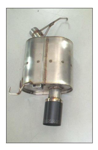
I. Support the muffler securely with a jack or a stand, locate the dimple on the stock pipe then cut the stock muffler as shown in **Figures 1 & 2**. Before cutting the stock muffler, hold DINAN muffler underneath stock muffler to verify the stock pipe will not be cut too short!
