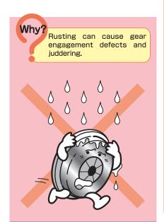
When changing the clutch, change it as a set of both the clutch disc and clutch cover.
