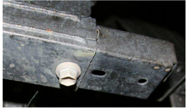
Figure 9 & 10 – Bumper beam extension and tow eye removal
