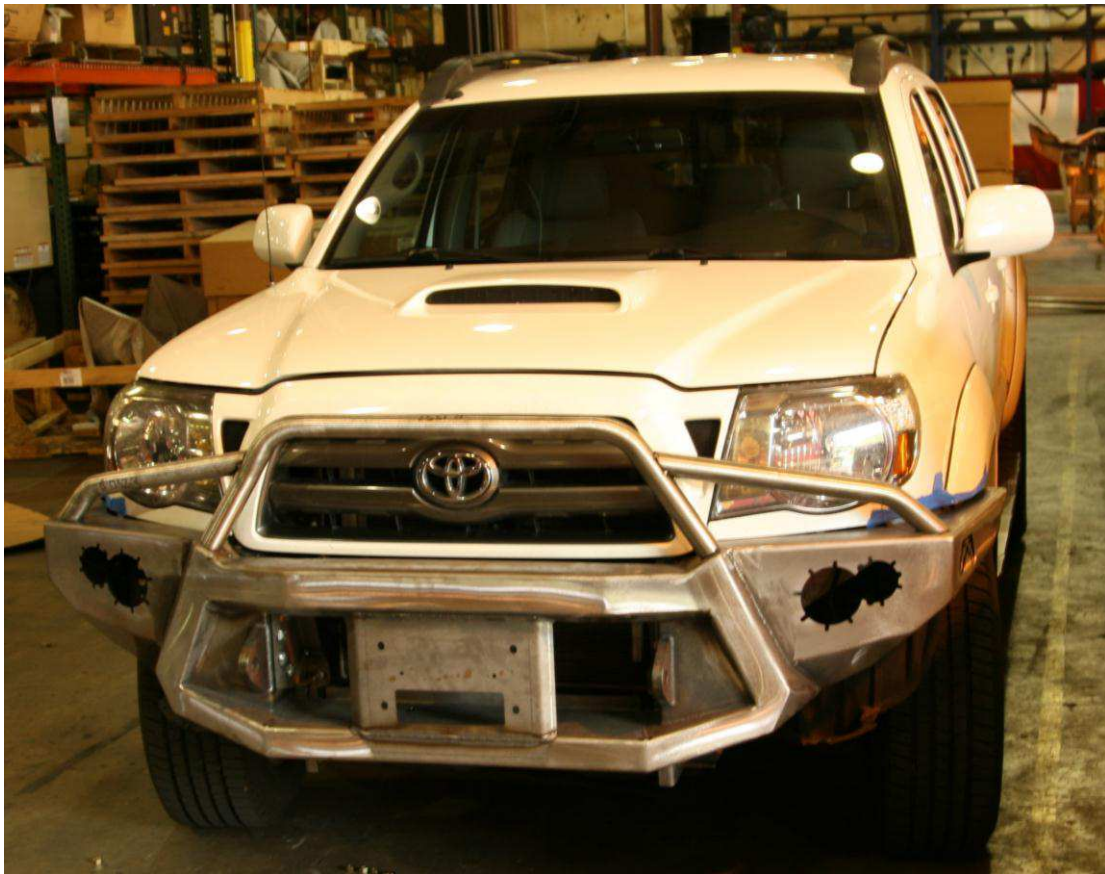
Figure 17 – Completed bumper installation (shown with PreRunner tube option)
