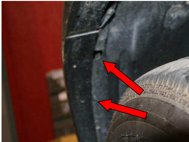
Figure 3 – Fenderwell fastener removal
