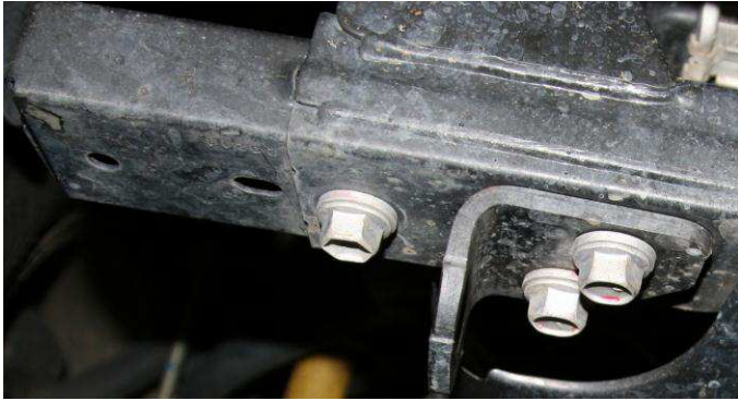
Figure 9 & 10 – Bumper beam extension and tow eye removal
