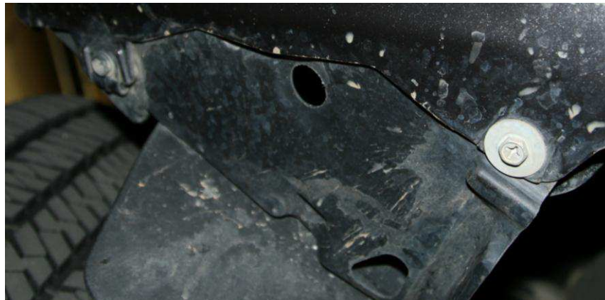
Figure 4 – OEM bumper cover screw removal
