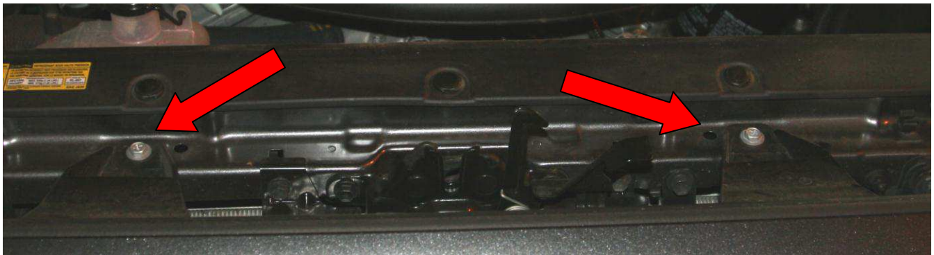
Figure 1 – Upper grill screw removal
