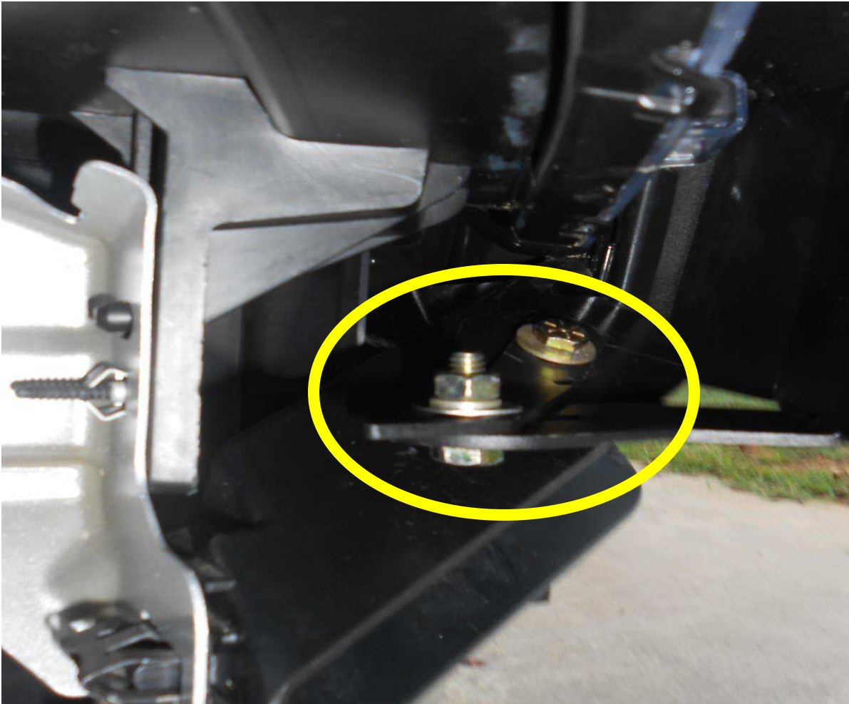
Figure 6c (bolts through mount points on valence mount and plastic of grill)
