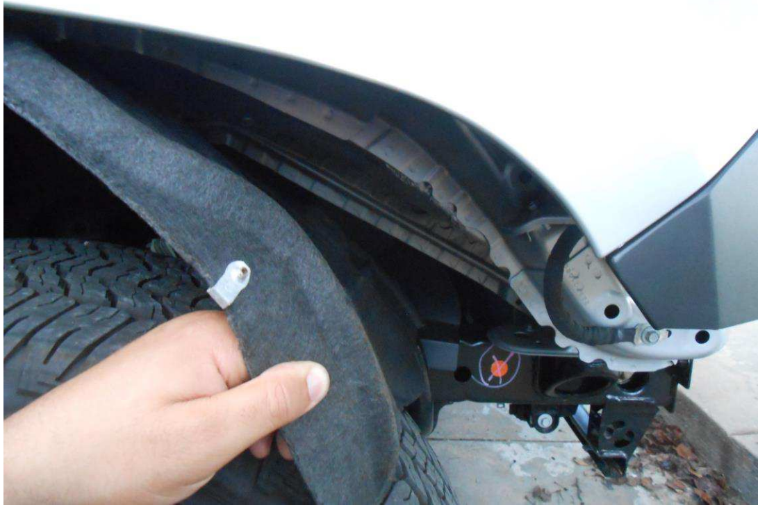
Figure 6a (wheel well liner pull back)
