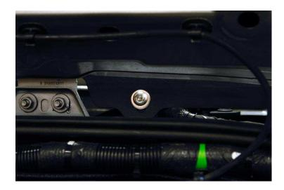
**6.** Center the Vi-Cowl on the windshield brackets then fully tighten the four pillar bolts.
