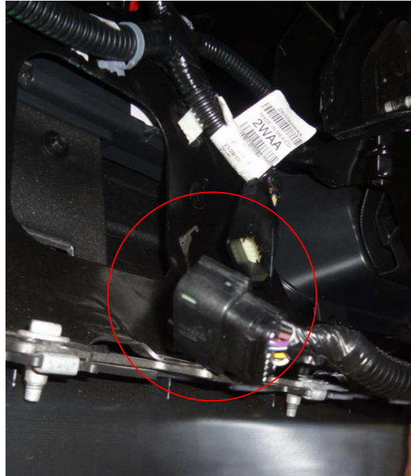
Figure 3(electrical harness disconnected)
