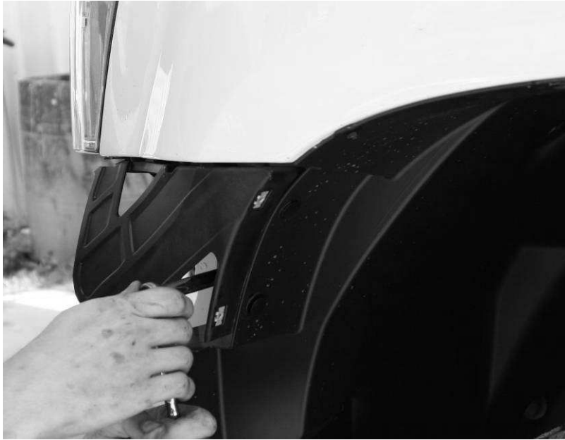
Figure 6 - Support Bracket Removal
