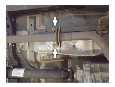
4. Disassemble factory exhaust wire hangers (x4) from isolators then remove system completely from vehicle.
