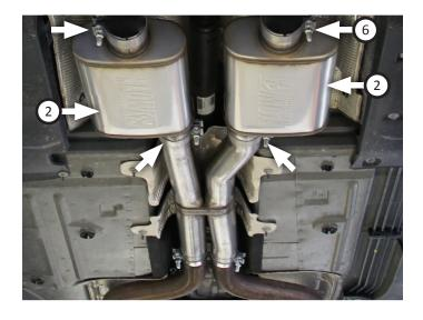
13. Transfer hangers from step 3 onto **right and left tailpipes (3, 4).** Connect them to mufflers, insert wire hangers (x2) into rubber isolators then rebolt rear hanger mounts to frame. Adjust tailpipes so their tips are level and centered in bumper cut-outs and tighten clamps just enough to allow for adjustment.
