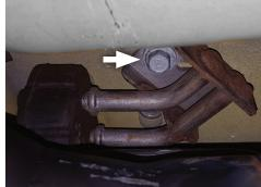
4. Carefully lower stands at vehicle rear and with help from an assistant, slide system back off the head pipes and lower system from vehicle.
