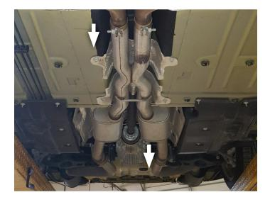
5. Remove nuts (x3) securing actuator to mounts on tailpipes. Then remove actuator and spring from mount on each tailpipe.
