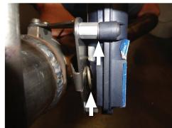
**NOTE:** Offset outlet pipe should be oriented to passenger side during install.
