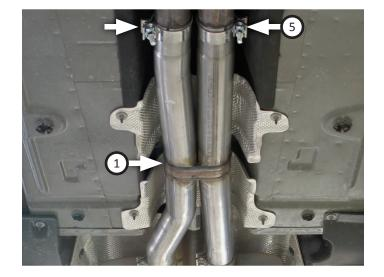
12. Place clamps (x4) (6) onto FFX mufflers (x2) (2) then connect it to scavenger pipe. Level parts then tighten clamps just enough to allow for adjustment.
