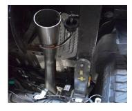
5. SLIDE EXIT PIPE #C USE CLAMP #F TO ATTACH PIPES TOGETHER. ROTATE EXIT PIPE TO ALLOW FOR PROPER CLEARANCE FOR TIP. DO NOT TIGHTEN.
