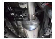
4. INSERT THE OVERAXLE TAILPIPE #B INTO THE OUTLET OF THE MUFFLER 1 ½" TO 2" INTO THE MUFFLER AND ATTACH USING CLAMP. INSERT WELDED HANGER INTO FACTORY RUBBER GROMMET. DO NOT TIGHTEN
