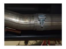
LAY OUT THE EXHAUST SYSTEM SO IT MATCHES THE DRAWING. MAKE SURE ALL PART NUMBERS ARE CORRECT, FOR AN EASIER REMOVAL OF THE FACTORY EXHAUST. CUT THE TAILPIPE JUST BEHIND THE FACTORY MUFFLER. LEAVE ALL RUBBER GROMMETS IN PLACE. USE WD-40 FOR EASIER REMOVAL OF FACTORY HANGER. UN **BOLT THE FACTORY CLAMP** LOCATED BEHIND THE FRONT RESONATOR AND REMOVE MUFFLER AND EXTENSION PIPE.
